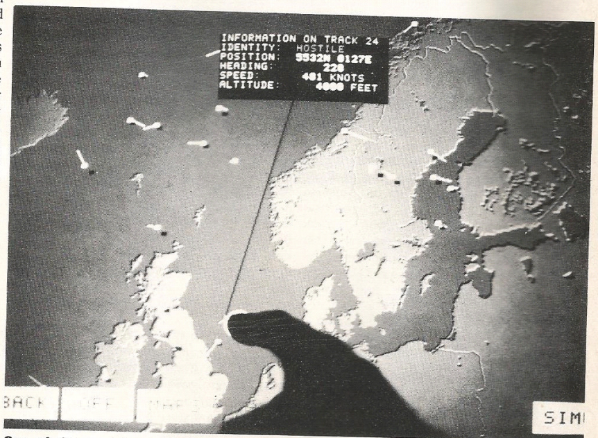
One of the air defence situation map presentations shown during the demonstration of EASAMS' new computer command and control system. 'Labels' for any displayed target can be called down by pointing to the target of interest
